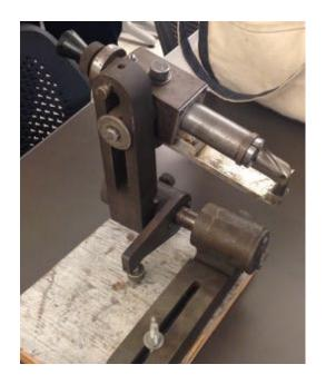
these parts. The drawings cost \$40 and include plans for the tool and it's accessories. Norm described how to use the tool to sharpen the end and flutes of end mills and also how to sharpen taps and he showed a fixture for sharpening 2-flute end mills he made from plans in HSM. Norm further described other accessories one can build to increase the tool's usefulness.
