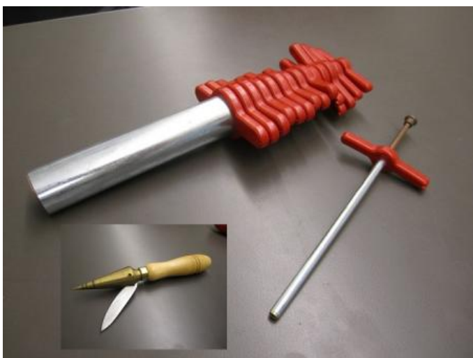
Cork boring set. Cutters nest for compact storage. Inset: Vintage sharpening tool for sharpening cutters.
