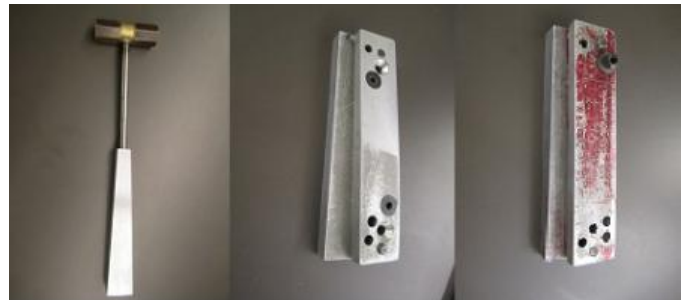
L: Brass hammer - Howard Weimer design, C&R: Fixtures used to machine handle.
