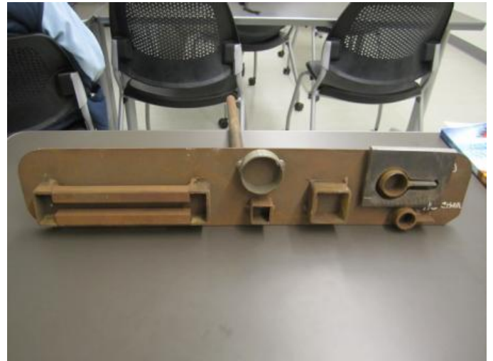
Home-made template plate containing various templates for use on Lewis Sullivan's Victor portable shape cutting machine. Note the finished piece in the upper right, resting on its pattern.
