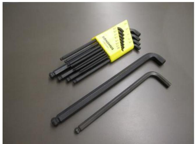
Top and Center: Low profile, ball end Allen wrenches; Bottom: Standard ball end Allen wrench
