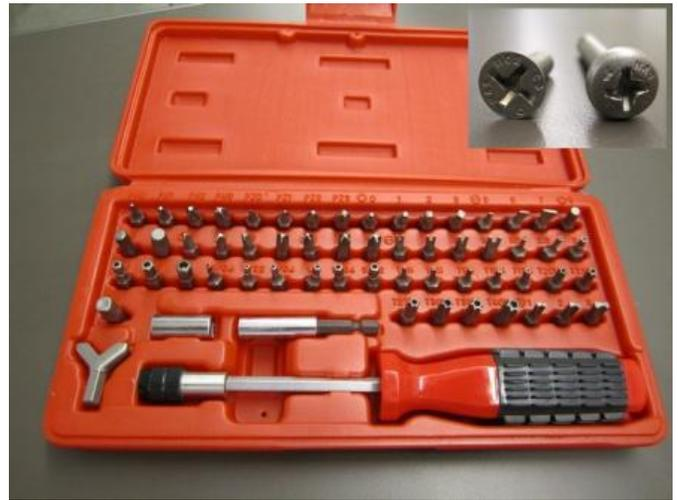
Grand Rapids Industrial Products driver bit set for tamperproof fasteners. Inset: Tamperproof screws.
