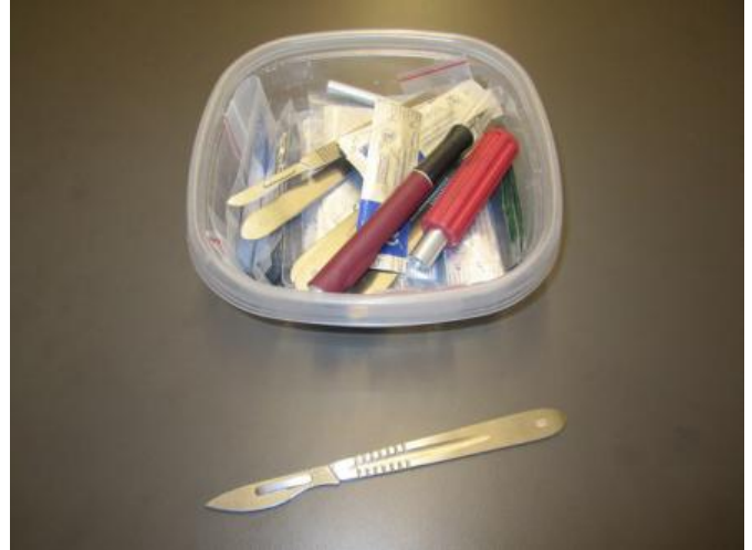
Assortment of scalpels, handy for hobby use and de-burring of plastic parts.
