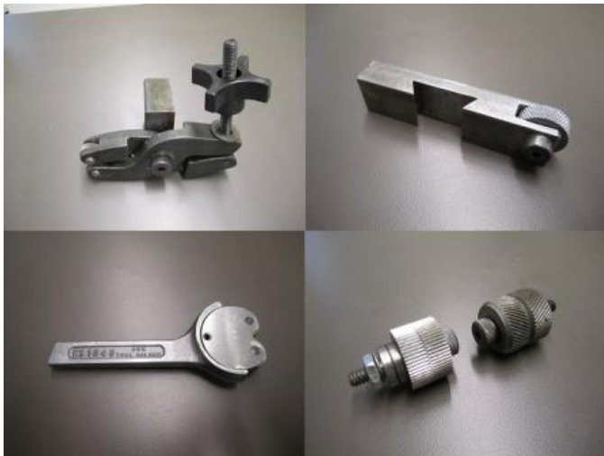
Norm Wells' assortment of knurling tools. Upper Left: scissor type Upper Right: "Bump Type" fits directly on Aloris style tool post. Lower Left: "Bump Type" fits in lantern style tool holder or quick change tool holders. Lower Right: Assorted knurl wheels.
