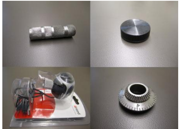
Norm Wells' knurling projects. Upper Left: sample knurls. Upper Right: knurled disk. Lower Left: replacement lock collar for USB camera. Lower Right: dial with knurl on beveled face.
