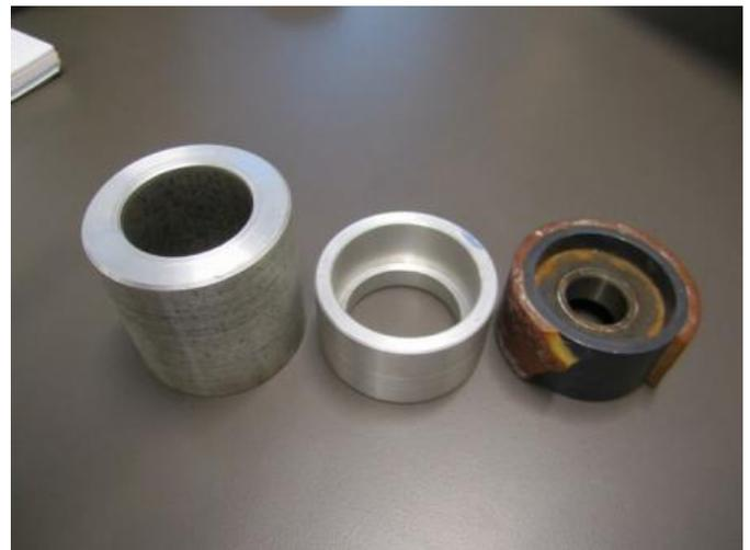
Bob DeVoe's replacement belt sander roller (Center) made from aluminum tubing (Left) to replace fire-damaged composite roller (Right.)
