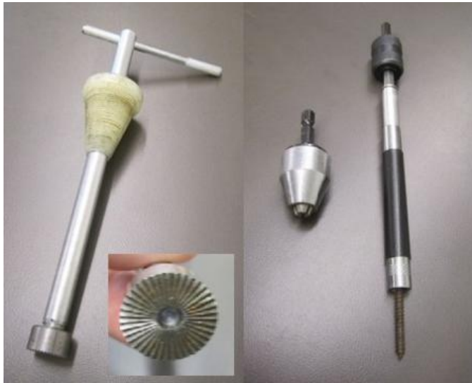
L: Seat Cutter R: Quick-Change Cordless Driver Accessories
