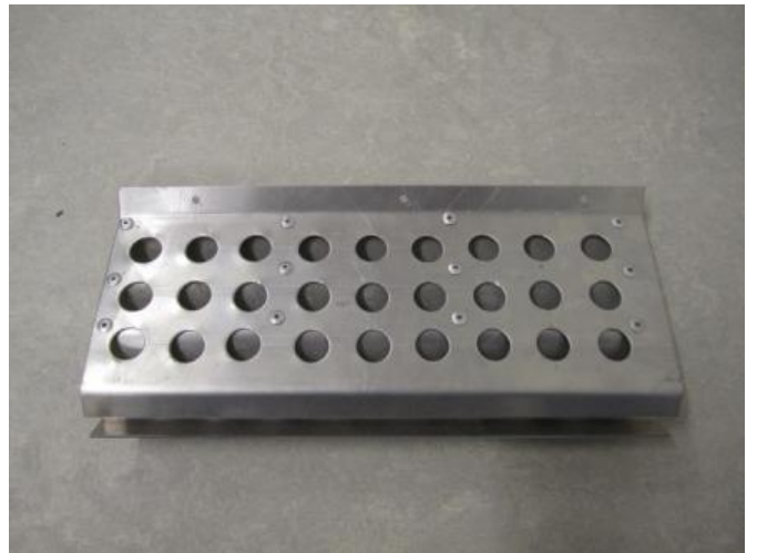
Lewis Sullivan's shop-made tooling rack made to fit between the vertical wall studs of his shop.
