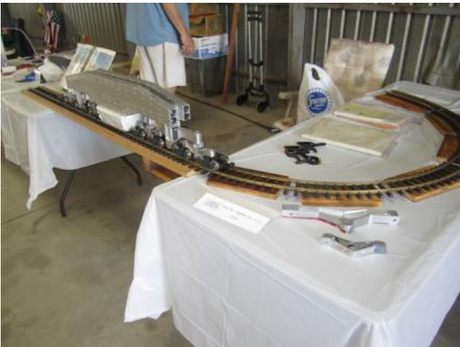
Phil Potter's model of a Schnabel Car. See lead ballast weight attached to the undercarriage.
