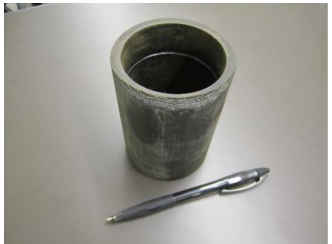
Worn composite main bushing from Lewis Sullivan's Ironworker.
