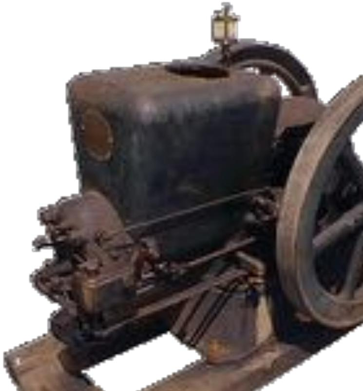
*A Fairbanks-Morse 6HP Model Z engine in as found condition. About 900 pounds with 190 cubic inch (3.1 liters) displacement*
